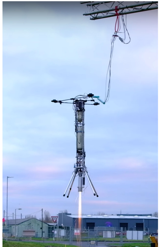
Figure 5: Gyroc VTVL rocket vehicle tethered hover, to tune control loops and explore system dynamics.
